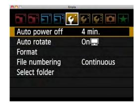
Auto Rotate. I set the camera to rotate images only when ingested to the computer, and not on the back of the camera. This way I can view vertical images using the camera's full LCD screen for a larger preview.
