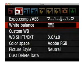
When shooting jpegs or video, it's crucial to set a custom white balance that is as accurate as possible. Jpegs and video clips are highly compressed files and don't allow for dramatic adjustments in color temperature, so you need to get it right in the camera. The box on the right shows how I set a custom color temperature. Take a test shot or use Live View mode to check your settings, and tailor the settings until the scene looks right.
