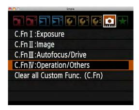
C.Fn IV-1, Shutter Button and Auto Focus. I select option 2 which moves autofocus controls to the AF-ON button rather than the shutter button. This way I can focus with my thumb on the AF-ON button, which I find more helpful when tracking a moving subject in AI Servo autofocus mode.
