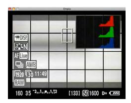
Another important setting in the Live View/Movie Function Setting pane is the Movie Recording Size, which selects both movie size and the frame rate. I commonly choose a 30p frame rate (30 frames per second) over the 24p frame rate as it allows me to capture better action clips of skiing etc. However many people prefer 24p, so check with your client for their needs first.
